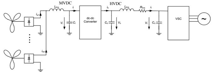
Figure 5: Application of dc-dc Converter in offshore wind farm
