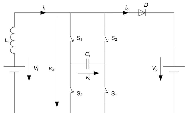
Figure 1: Simplified structure of the step-up converter
