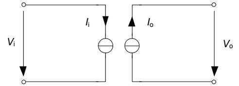
Figure 3: Equivalent circuit diagram for the step-up converter
