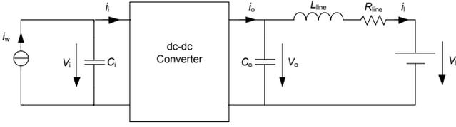
Figure 6: Converter model in order to connect an offshore wind farm to a VSC
