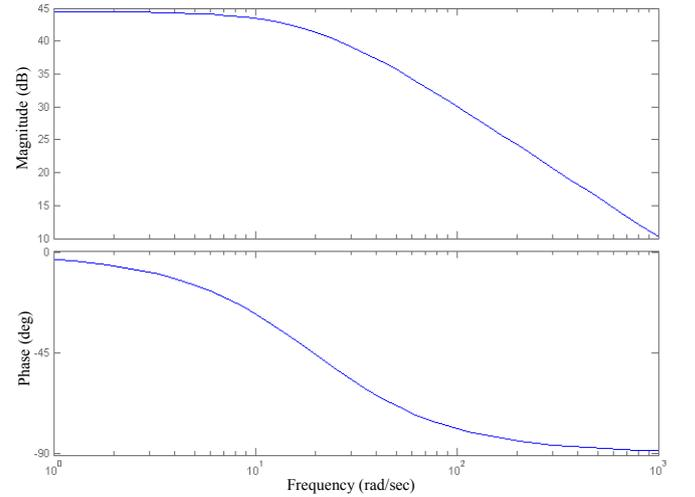
Figure 8: Bode plot of the simplified system
