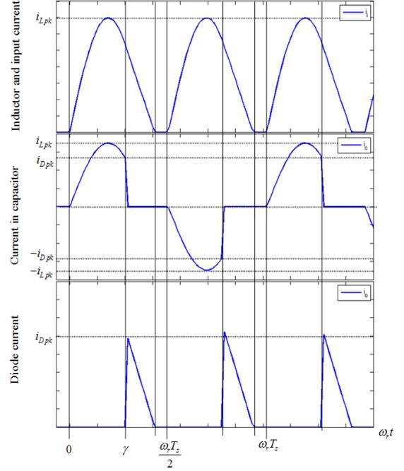
Figure 2: Ideal steady state waveforms for the step-up converter
