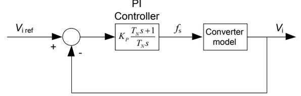
Figure 4: Control structure of the system
