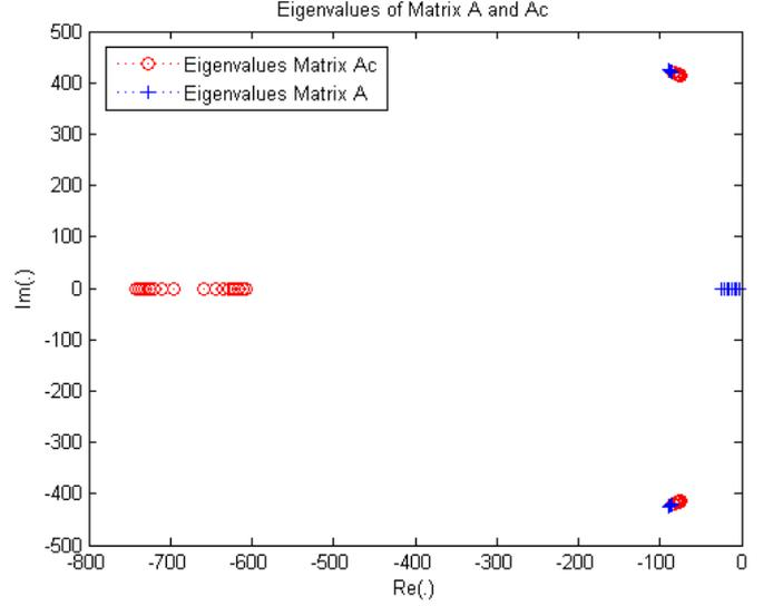
Figure 10: Eigenvalues of the closed and open loop system
