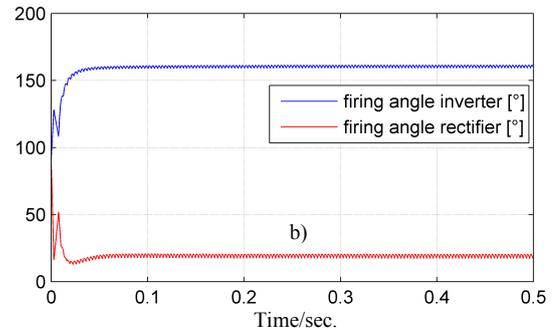
Figure 10: Firing angles of the HVDC system with a) the classical controller b) the decoupling filter controller
