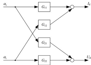
Figure 3: Structure of the simplified HVDC Model
