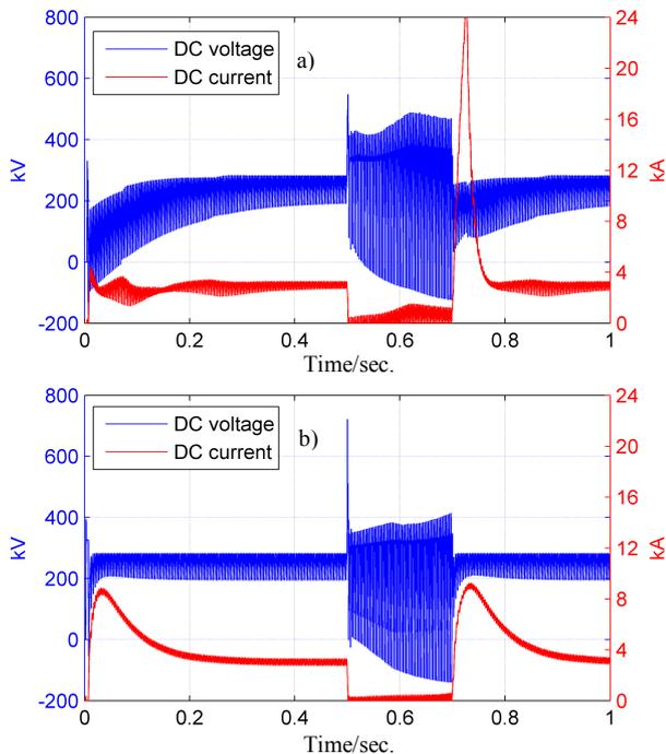
Figure 11: 50 % voltage jump from  $t = 0.5$  sec to  $t = 0.7$  sec applied to the inverter AC side of the HVDC system with a) the classical controller b) the decoupling filter controller
