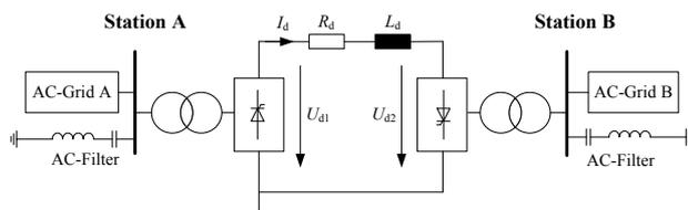
Figure 1: Schematic design of a six pulse HVDC system
