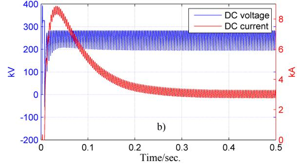
Figure 9: Power-up process of the HVDC system with a) the classical controller b) the decoupling filter controller
