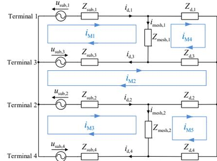
Figure 10: Mashed HVDC system represented as connection of subsystems (with  $Z_{\text{mesh},n}$ )
