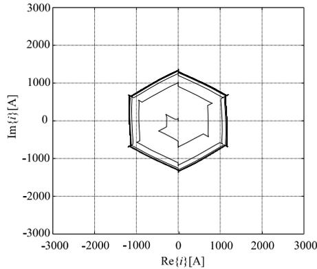
Figure 16: Grid current space phasor of terminal 1
