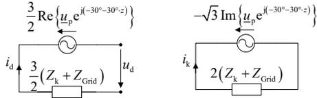
Figure 6: Real and imaginary part network for COM in general
