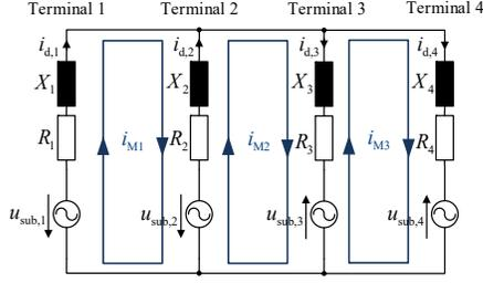
Figure 9: Radial HVDC system represented as a connection of subsystems (without  $Z_{\text{mesh},n}$ )
