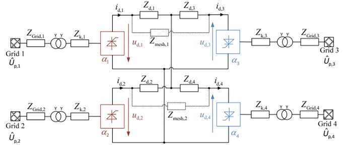
Figure 8: Configuration of a 4-terminal HVDC System
