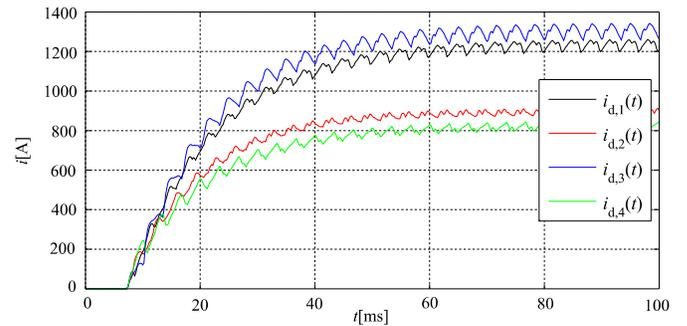
Figure 12: DC currents of the analytical model
