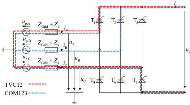
Figure 1: Line commutated six-pulse converter
