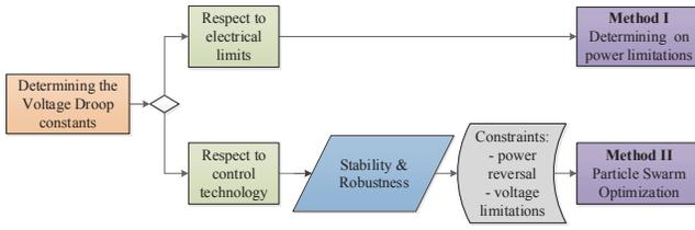
Fig. 5. Methods for the determination of the droop constants with emphasis on robustness
