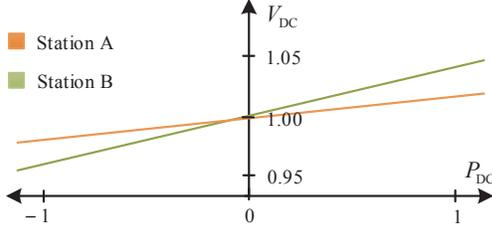
Fig. 2. Example of a Voltage Droop Control characteristic for two stations [7]
