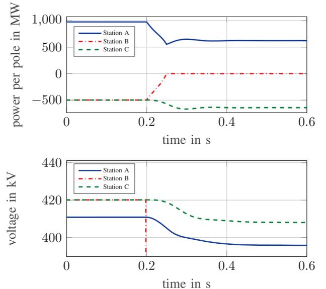
Fig. 7. Simulation of operating point I – Determination of the droop constants with method I
