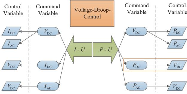
Fig. 1. Overview and classification of the Voltage Droop Control with highlighting of the used approach [5]
