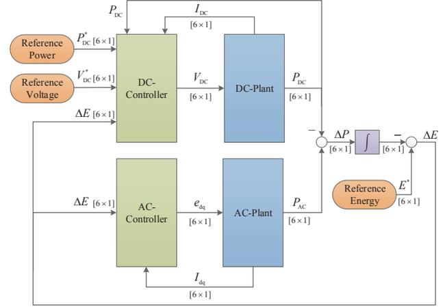
Fig. 4. Block Diagram of the developed MTDC Model with its control
