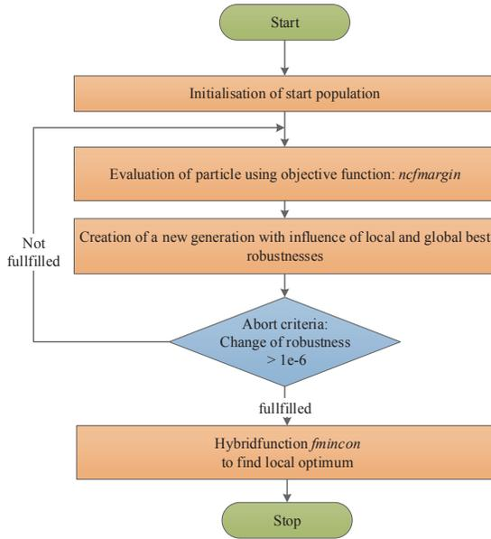
Fig. 6. Flow chart of the determination process of the droop constants with emphasis on robustness
