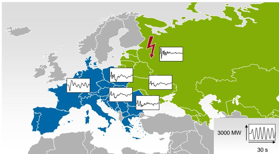
Figure 3: Profiles of wide-area power oscillations after a severe disturbance in the IPS/UPS
