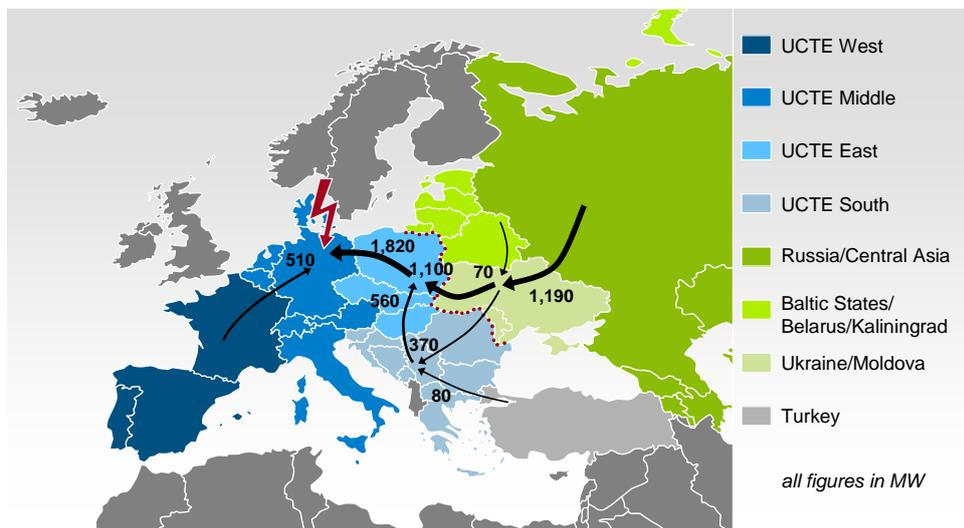
Figure 4: Control power flow after an outage of 3000 MW in UCTE
