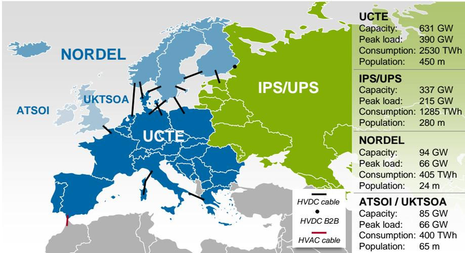
Figure 1: Synchronous systems in Europe and key figures (2008)
